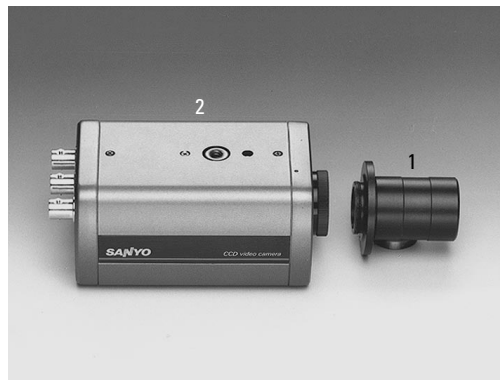
Fig. 79 Adaption of the front port for TV camera 1 TV adapter 0.63x, 2 TV camera with c-mount thread
